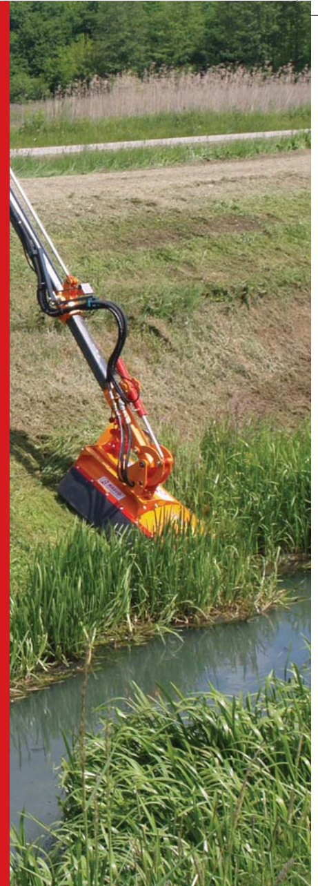
mowing head with mid-weight blades
